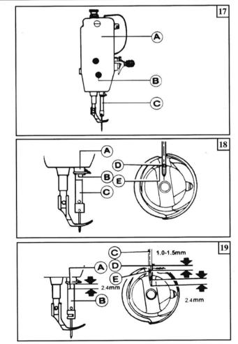
The motive relation between retating hook and needle affects the sewing quality. Standard timing relation is: turn the balance wheel to locate needle bar to its lowest position, and loft back 2.4mm the rotating hook point (D) should be coincides with needle center line (C), and hook point (D) is 1.2mm above the upper edge (E) of needle eye.
