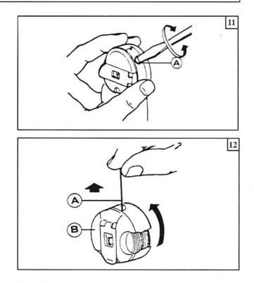
adjusted by changing tension of the thread take-up spring sewing range of the thread take-up spring tension of tension disc. and the position of thread guide.
