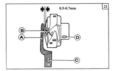
The projecting flange of the position bracket (A) should be engaged in the notch(B)of the bobbin case holder, and maintain a clearance of 0.5~0.7mm between projecting flange top and the bottom of notch while installing.
