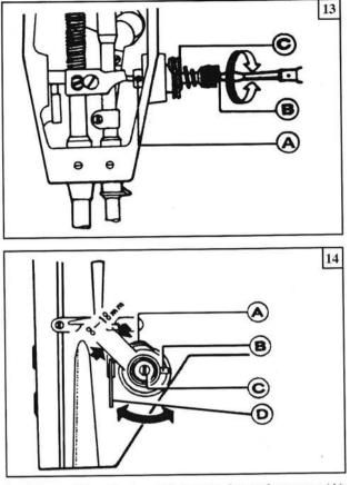
by 1/2 turn. After adjustment, tighten tension stud set screw (A).
