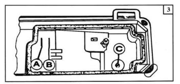
machine.Turn balance wheel slowly to see if there is any obstacle, collision and uneven resistance between parts. If there is, adjustment should be done before operation.
