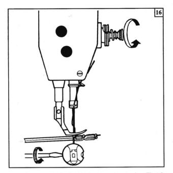
screw drive to make the bobbin thread get less tension (Fig 16)(c) Other abrormal stitches as shoewn in Fig.15(d)(e), adjustment can be made which reference to the above methods.
