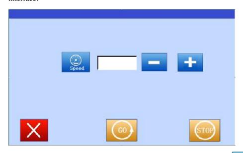
Press to increase or decrease the speed, also can press to set the speed directly(range:100-1000). After set, press to start, and press to stop, then press to return to the equipment maintenance interface.
