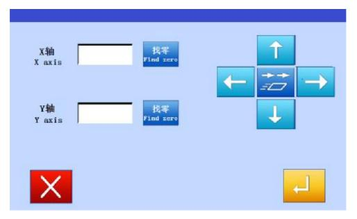
Press directional keys to adjust X,Y origin, make sure the needle is in the center of 4 directions "front, back, left and right". It is better not to adjust the X,Y origin directly by
