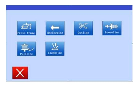
Press each button, the relative electromagnet will pull and release.
