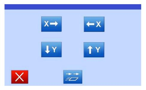
Press each directional keys, the X,Y stepping motors will move quiet and at steady speed. Press to speed up or slow down the speed.
