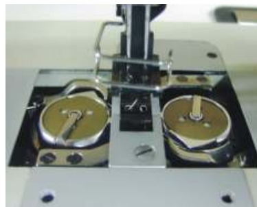
Two Large Horizontal Hooks and Bobbins
