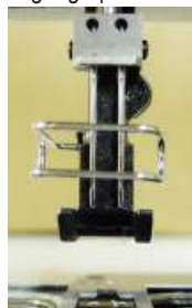
Detail of twin needles showing high presser foot lift
