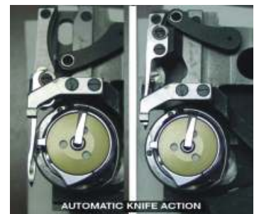
Auto Thread Cutter shown engaged and retracted
