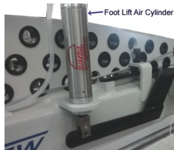
733R-6 machines have air cylinders to drive the footlift and reverse
